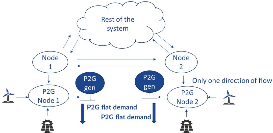
Figure 38 - Simplified diagram of P2G modelling
