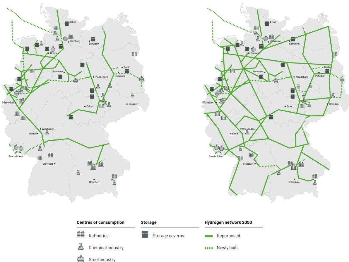
**Figure 17: Hydrogen Network 2030 and 2050 of FNB Gas (Source: [2030](#), [2050](#))**
