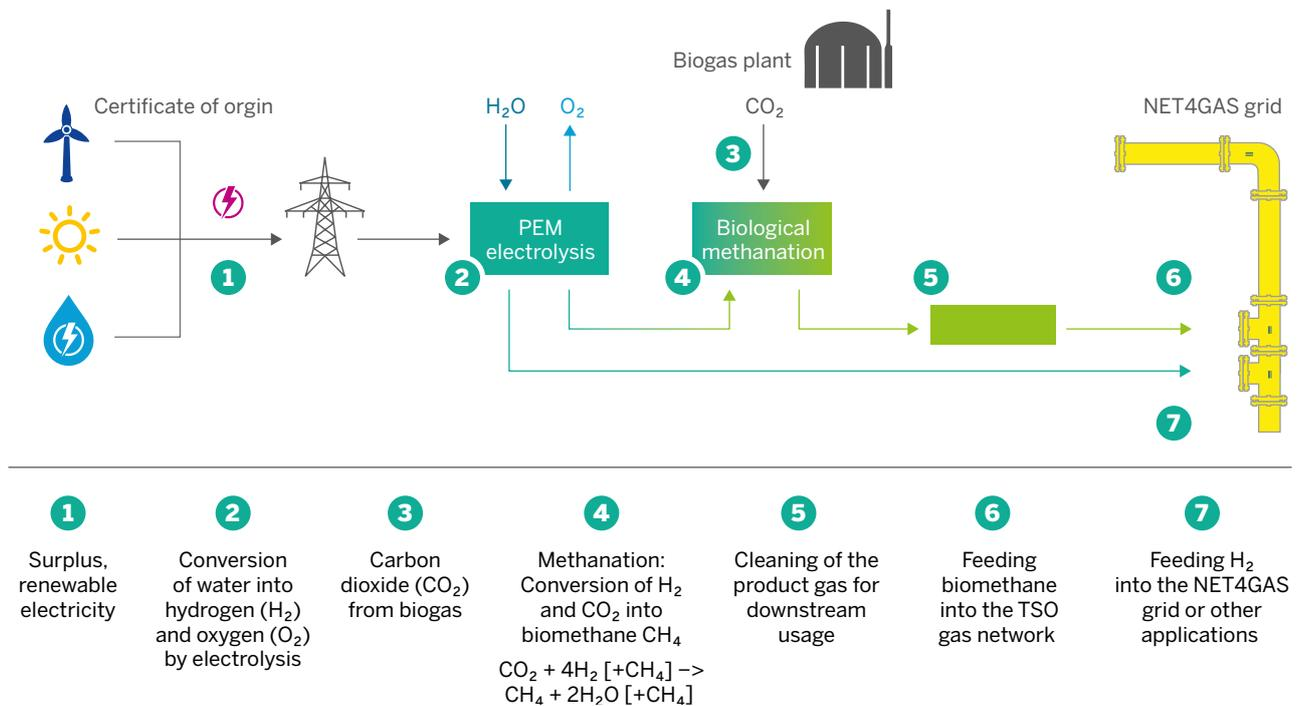
Figure 9: Schematic description of the prepared Power-to-Gas facility (Source: NET4GAS)
