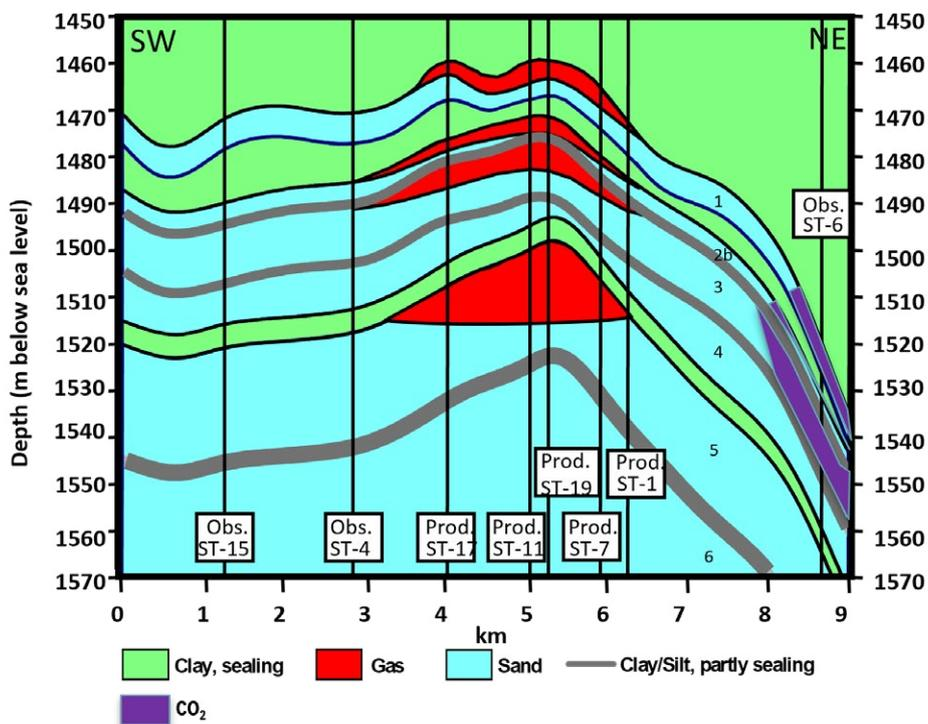
Figure 13: Schematic of underground CO<sub>2</sub> storage in Denmark (Source: Gas Storage Denmark)
