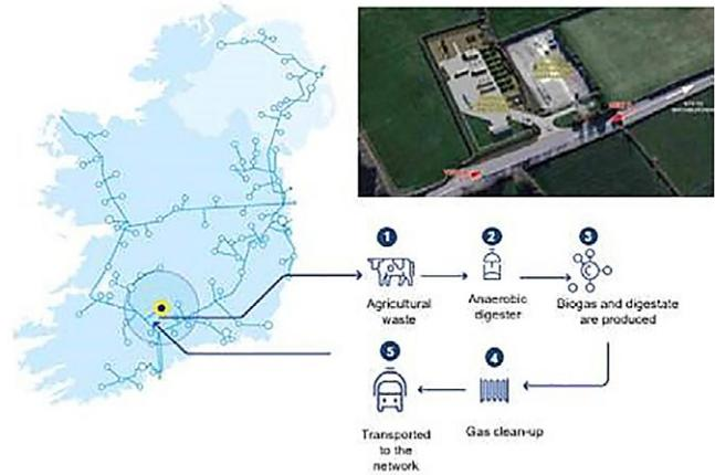
Figure 25: Overview of Centralised Grid Injection Concept, Gas Networks Ireland
