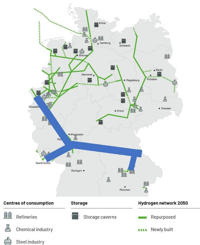
Figure 20: Schematic representation of the envisaged pipeline sections (blue) in the Hydrogen Network 2030 of the FNB Gas
