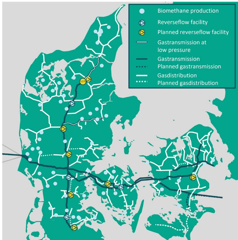
**Figure 10: Existing and planned reverse flow and biomethane production facilities in Denmark**
