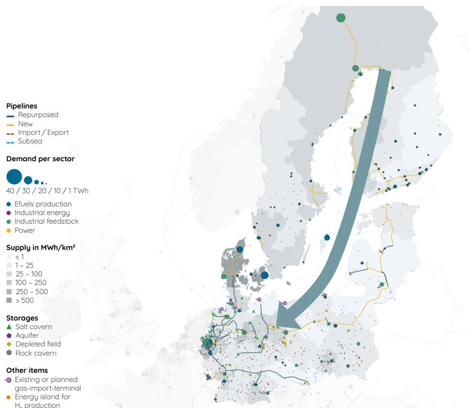
Figure 23: Nordic-Baltic Hydrogen Corridor (Source: European Hydrogen Backbone report)
