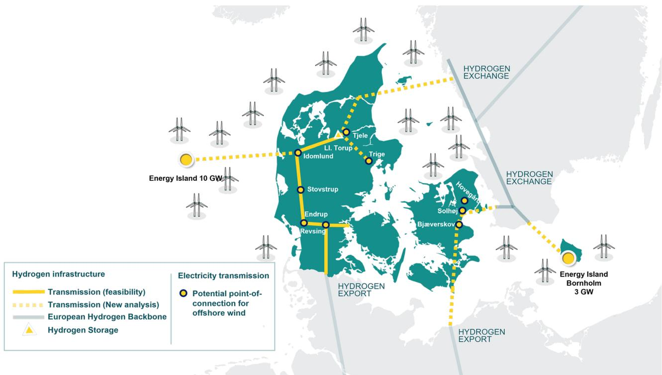
Figure 12: Example of possible hydrogen infrastructure in Denmark (Source: Energinet)
