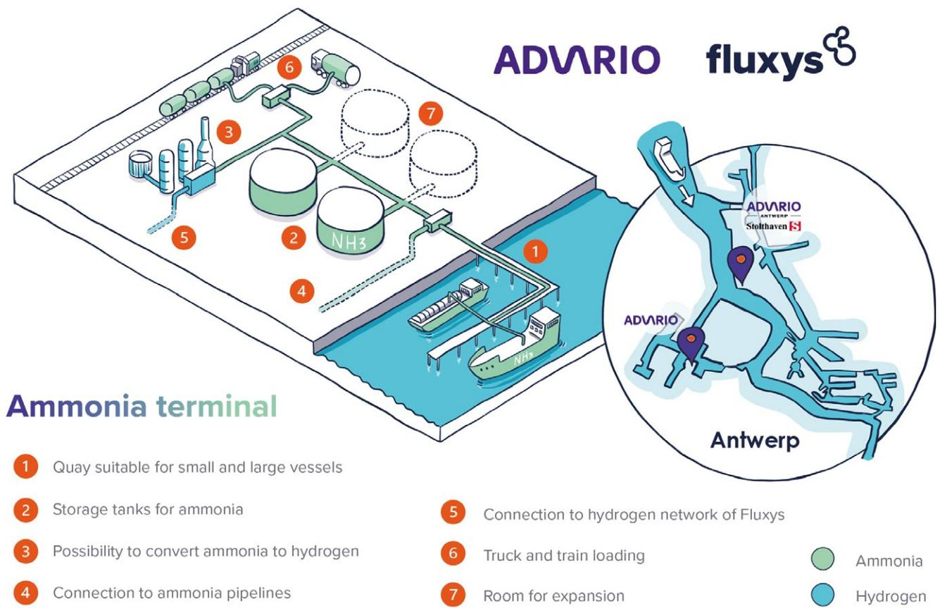
Figure 4: Illustration of the ammonia terminal (Source: Fluxys)
