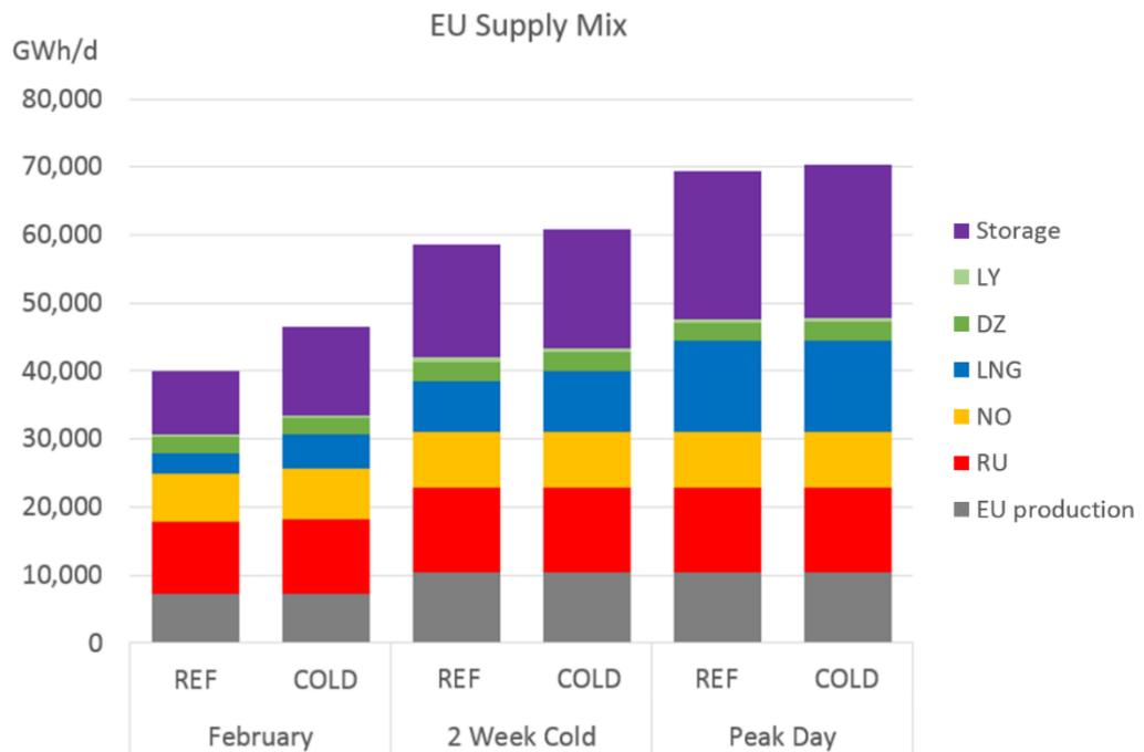
**Figure 10: Comparison of supply mixes in February vs high demand situations**
